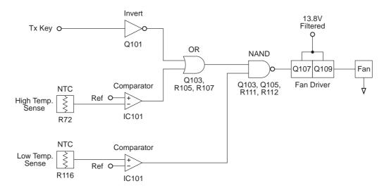
Figure 2.3 T889 Fan Control Logic Diagram
