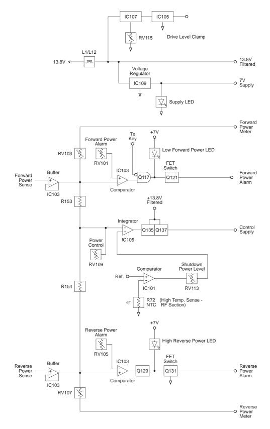
Figure 2.2 T889 Control Circuitry Block Diagram
