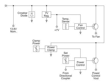
Figure 2.4 T889 Power Supply & Regulator Circuitry Block Diagram
