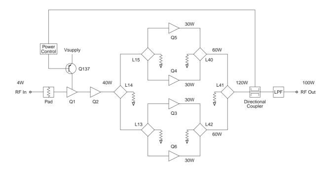
Figure 2.1 T889 High Level Block Diagram
